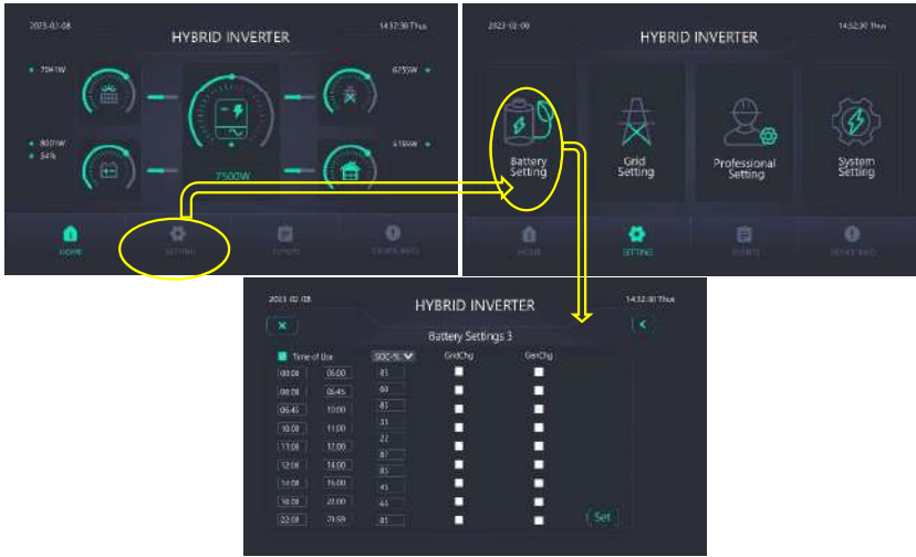
Figure 4.3 Schematic diagram of setting time curve
