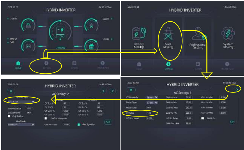
Figure 3.17 Intelligent Load and CT Ratio Setting Path
